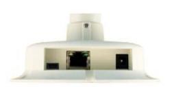
EtroLink™ Config Port 10/100Mbps Ethernet Port 12V DC Power
